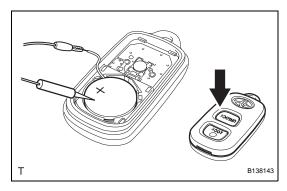
(1) Remove the battery (lithium battery) from the transmitter.
